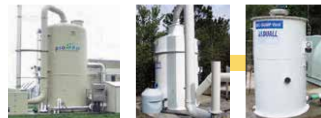
Biotrickling Filter Removing Odors
