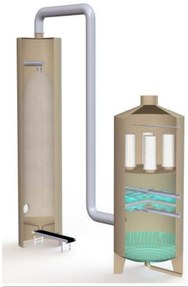
Figure 1. Dual-stage wet scrubber.
