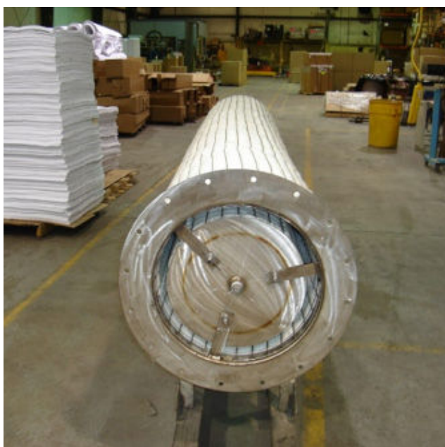
Figure 5. Mist eliminator designed by CECO.
